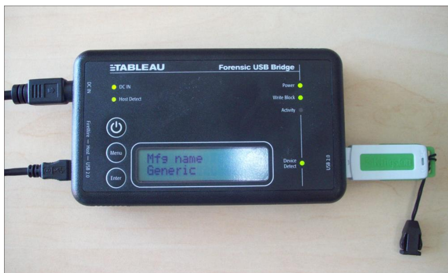
Figure 39: Tableau USB write block with USB as the source drive
